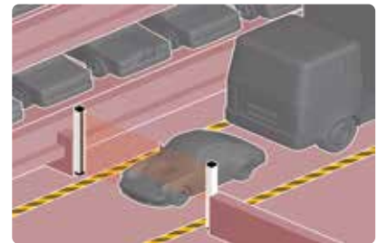
Detection of overall dimensional limits of vehicles in automated parking garages
